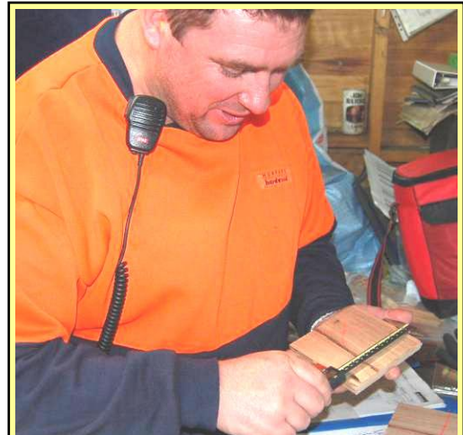
A quality control officer measures the width of a milled board with his Vernier calipers, and checks that it is within the tolerances shown in the specifications.
