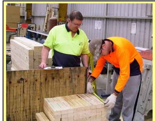
A supervisor oversees his production worker checking the tolerances on a special order of cut-to-length components.
