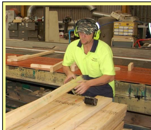
A quality control officer removes a length of timber that has been graded incorrectly.
